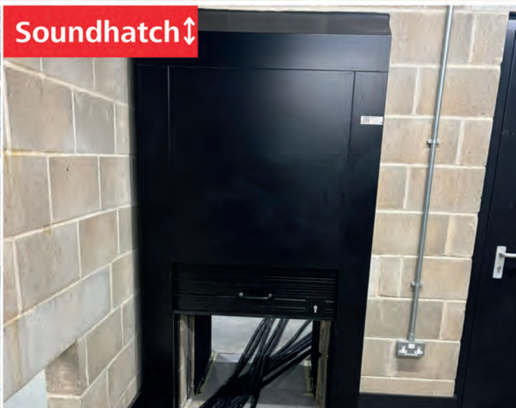
Vertically lifting counterbalanced cable access hatch Rw30dB, Rw31dB, Rw53dB
